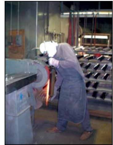
Finishing for most motorcycle parts begins with polishing, either by hand or on one of VCP's three robotic cells.
